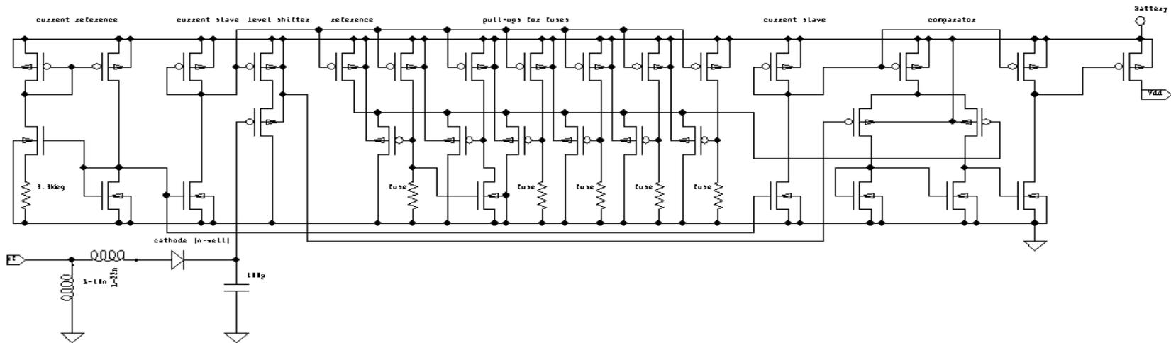
The voltage provided by the diode is compared with an internal reference voltage, and activates a switch when the rectified voltage exceeds the internal reference value. The sensitivity of this circuit is adjusted by changing the internal reference voltage.
