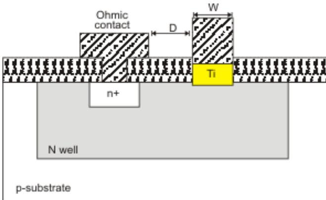
Figure on the left shows cross-sectional view of the Schottky barrier diode. Here the Schottky diode contact width is  $W$ , and the separation between the Schottky contact and the Ohmic contact is  $D$ .
