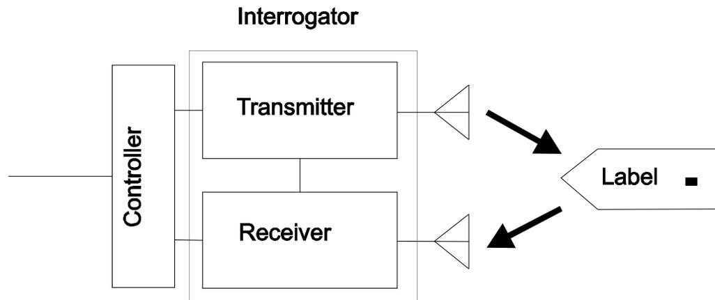
Here a transmitter of interrogation signals which is contained within an interrogator communicates via electromagnetic waves with an electronically coded label to elicit from the label a reply signal containing useful data characteristic of the object to which the label is attached. The reply signal is detected by a receiver in the interrogator and made available to a control system.
