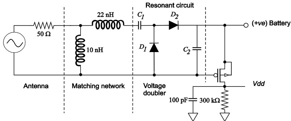
In this proposal a p-channel FET was used as a switch to control the power supply to a labels control circuits and can be triggered by the incident RF radiation on the antenna. Thus the power generated and amplified by the diode resonance can be utilized to turn a p-channel FET from an off state to an on state.
