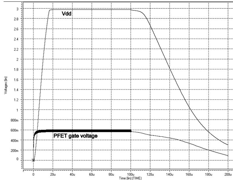
Simulated results for the turn on circuit implementation using HSPICE diode model for the fabricated CMOS Schottky diode
