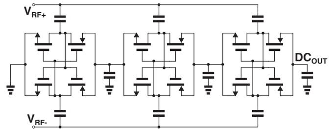
Fig. 4. The 3-stage differential-drive rectifier schematic.
