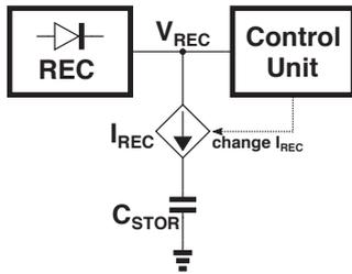
Fig. 2. A conceptual diagram of the proposed design, where the control unit regulates the output voltage of the rectifier  $V_{REC}$  by changing the output current of the rectifier  $I_{REC}$ .
