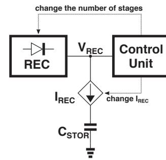
Fig. 7. Conceptual model of the improved design, where the control unit regulates the output voltage of the rectifier  $V_{REC}$  by changing the output current of the rectifier  $I_{REC}$  and it also reconfigures the number of stages within the rectifier as a function of input power.
