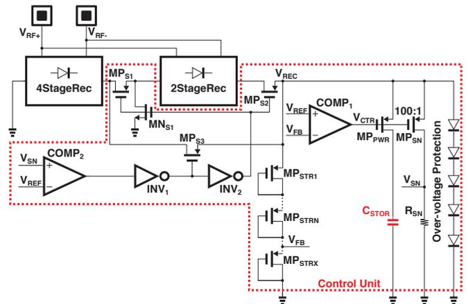
Fig. 8. Circuit realization of the proposed energy harvester.
