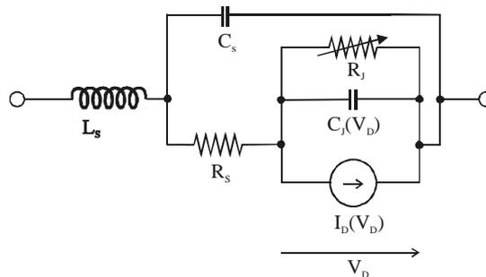
Figure 3: High frequency diode model
