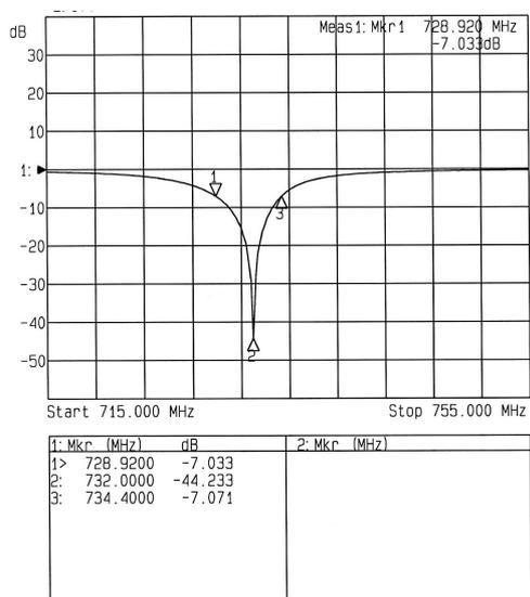
Figure 6: Low power Q: the return loss plot obtained with the network analyser output power level set to -35dBm indicates a low power Q of approximately 130.
