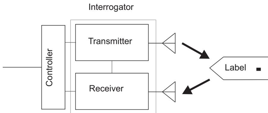
Figure 1: Illustration of an RFID system.
