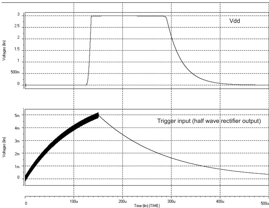
Figure 11: Simulated results for the low power turn on circuit implementation in Figure 9 using a HSPICE diode model for the fabricated CMOS Schottky diode.
