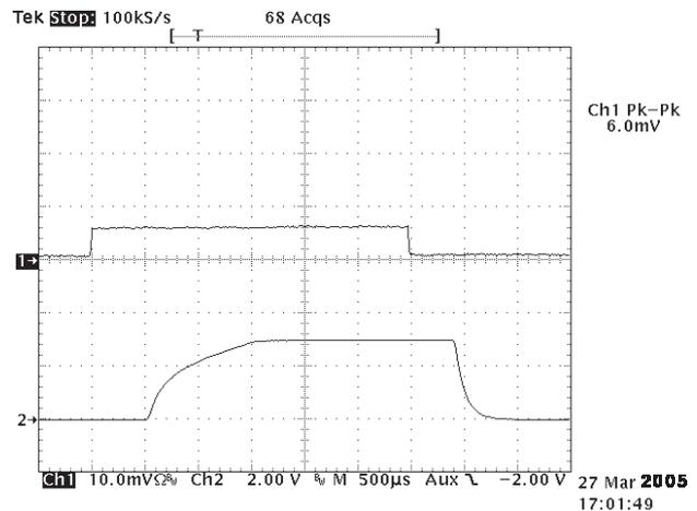
Figure 13: Response of the circuit to a 6mV rectified d.c voltage.
