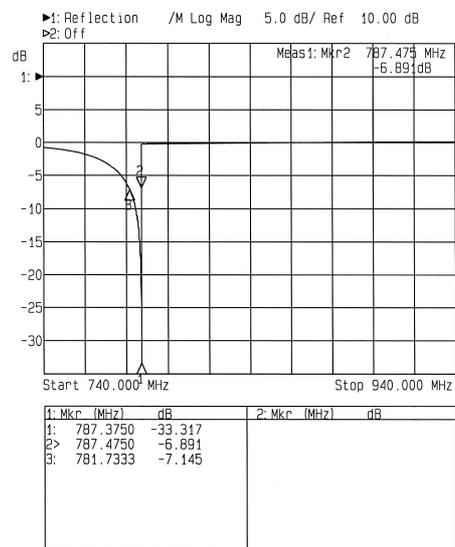
Figure 7: High power Q: the return loss plot obtained with the network analyser output power level set to -19dBm depicting the non-linearity of the circuit response.
