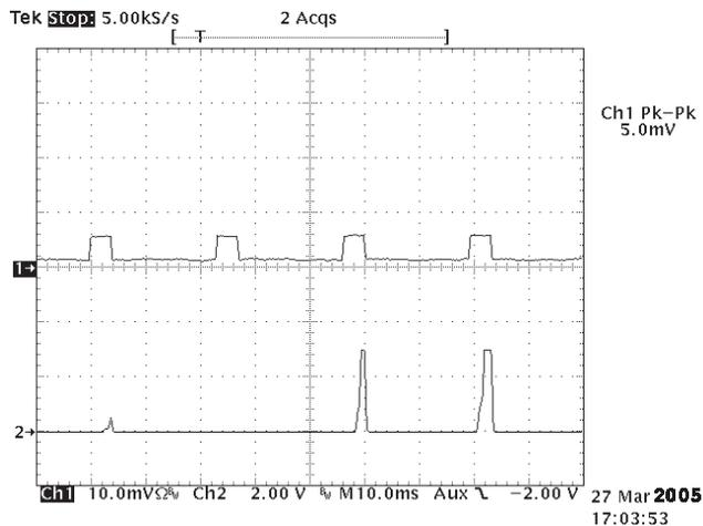
Figure 12: Response of the circuit to a 5mV rectified d.c voltage
