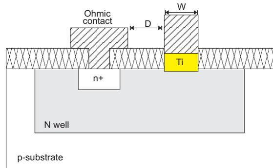
Figure 8: Cross-sectional view of the Schottky barrier diode. Here the Schottky diode contact width is  $W$ , and the separation between the Schottky contact and the Ohmic contact is  $D$ .
