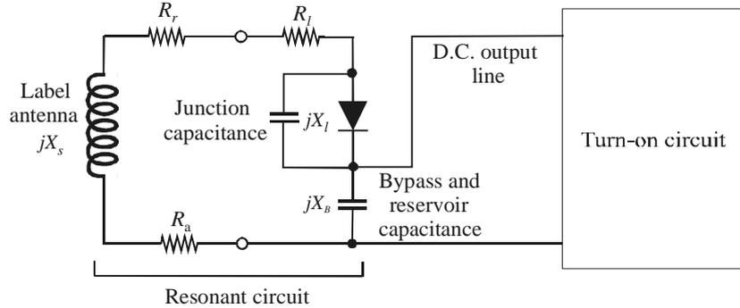
Figure 2: label rectification circuit
