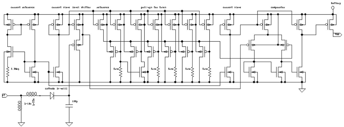
Figure 10: A turn-on circuit based on rectified input voltage of 5 mV d.c. output based on a internal reference voltage with trimmable sensitivity.
