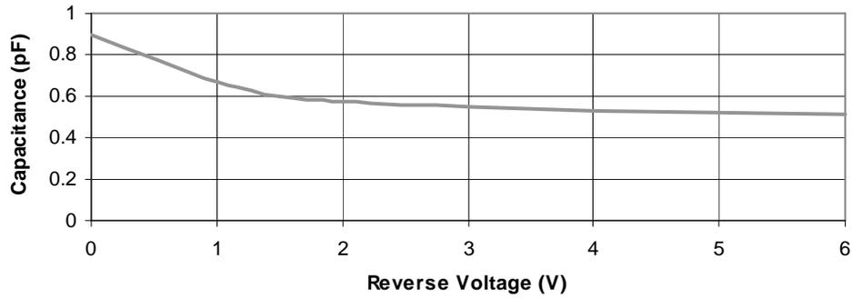
Figure 4: Junction capacitance: Variation of the diode junction capacitance as a result of the reverse voltage
