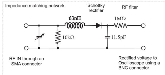
Figure 5: Simple diode rectification circuit
