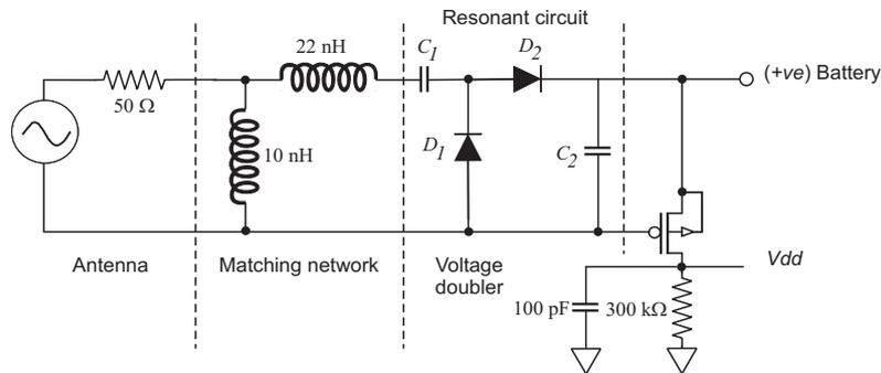
Figure 15: Turn on circuit implementation used in an HSPICE simulation.
