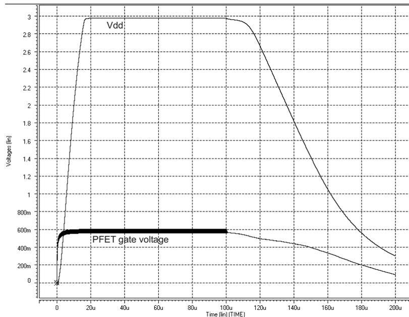
Figure 16: Simulated results for the turn on circuit implementation using HSPICE diode model for the fabricated CMOS Schottky diode.
