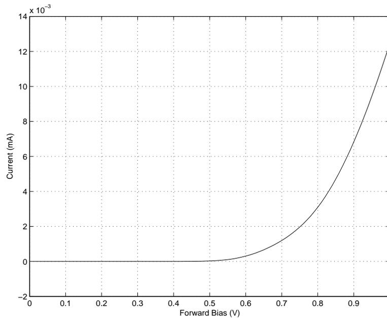
Figure 9: Measure IV curve of the CMOS Schottky barrier diode
