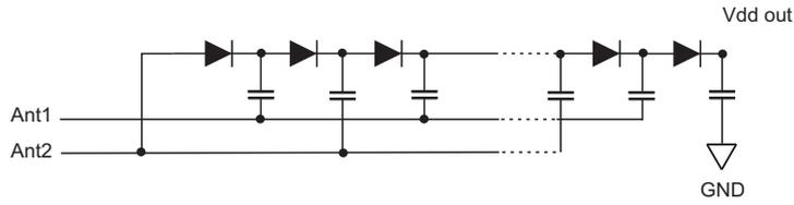
Figure 8: A multi-stage multiplier schematic based on the Schottky Barrier Diode (SBD).
