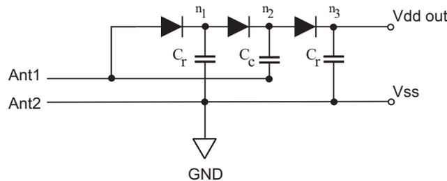
Figure 7: A novel rectifier/multiplier topology using the SBD, based on Dickson's design.
