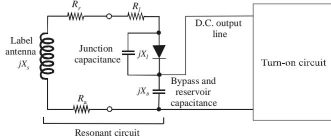
Figure 2: A simple overview of a label rectification circuit
