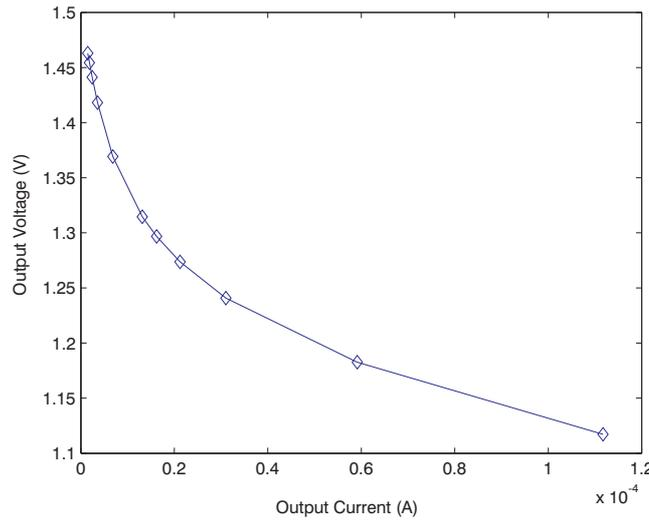
Figure 9: The output voltage as a function of the output current for a two stage charge pump.
