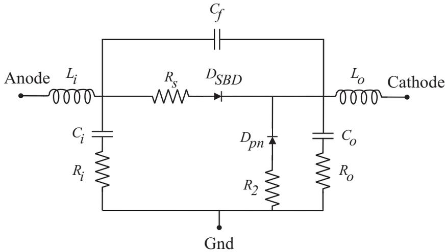
Figure 6: Equivalent circuit model of a Schottky Diode on standard CMOS process outlined in [13].
