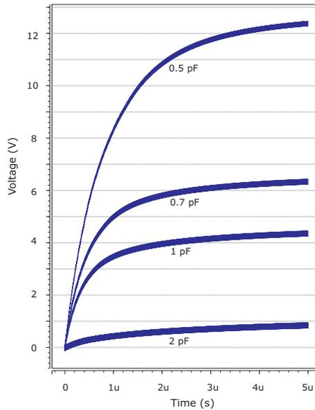
Figure 14: Effects of junction capacitance on the output voltage.
