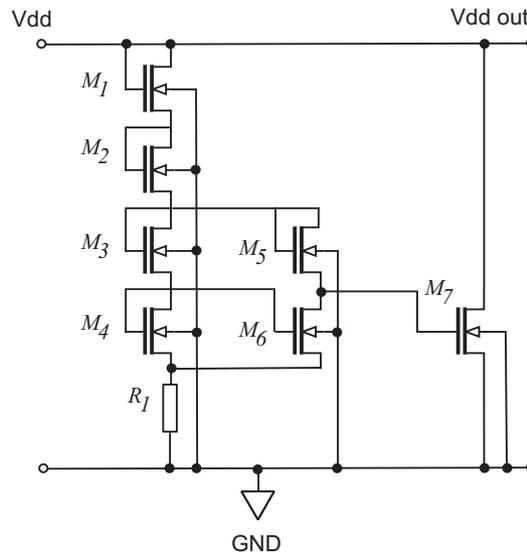
Figure 15: circuit schematic of shunt regulator.
