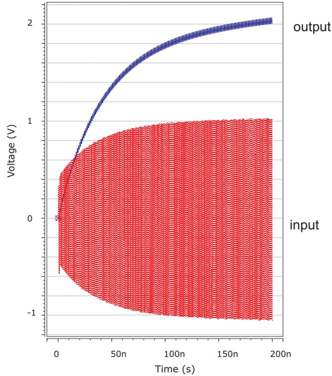
Figure 10: Plot of input and output of a single stage voltage multiplier circuit.
