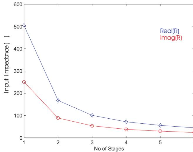
Figure 13: Plot of input impedance vs. number of stages in the rectifier structure.
