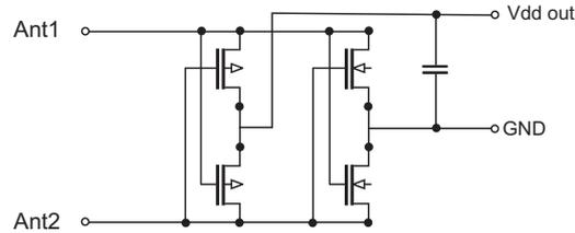
Figure 3: MOS bridge rectifier network.
