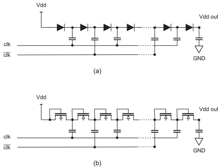
Figure 5 Functional diagram of (a) diode based Dickson charge pump and (b) a functional diagram of a traditional Dickson charge-pump.
