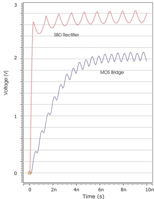
Figure 4: Comparison of the response time of a SBD diode with a MOS bridge rectifier circuit.
