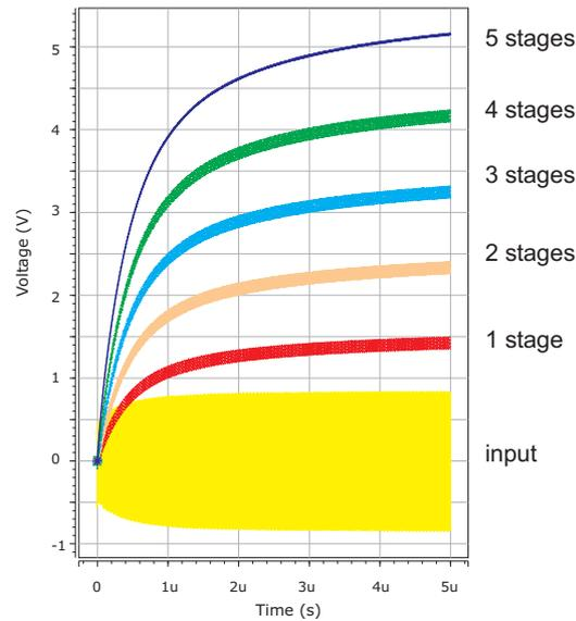
Figure 11: Comparison of output voltage versus input from 1 to 5-stage case.
