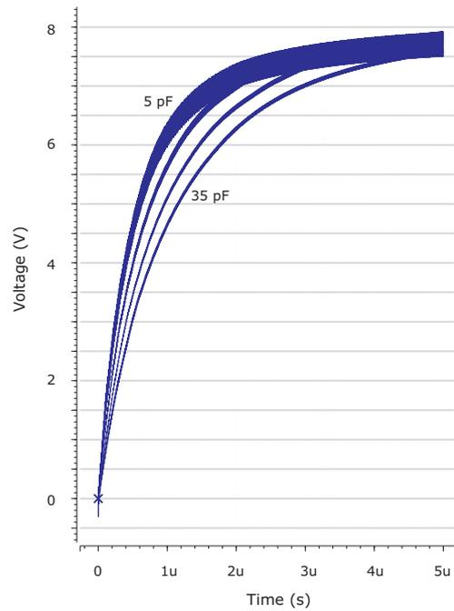
Figure 12: Effects of  $C_c$  and  $C_r$  on the output voltage.
