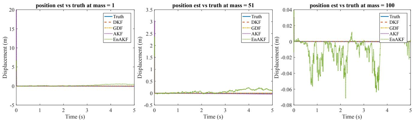
Fig. 5. Displacement estimations based on GDF, AKF, DKF and EnAKF versus truth values of a set of representative masses.
