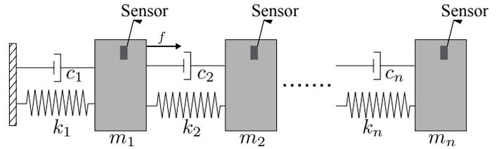
Fig. 1. An  $n$ -DoF structural system.
