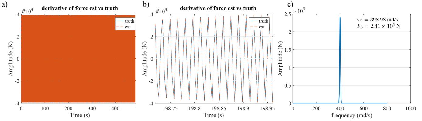
Fig. 2. Estimated values of  $\hat{d}_k = \frac{F_0 \omega_0 \Delta t}{m_1} \cos(\omega_0 k \Delta t + \phi_0)$  versus its ground truth: a) over 500 s; b) over a small window for clarity. c) Estimated force parameters based on  $\hat{d}_k$ 's values.
