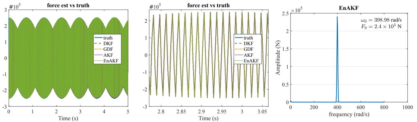
Fig. 4. Estimated values of  $f$  based on GDF, AKF, DKF and EnAKF versus its ground truth: a) over 5 s; b) over a small period for clarity. c) Force parameters estimated from  $\hat{f}$  values (since four methods result in the same estimated parameters, only one graph is plotted here).
