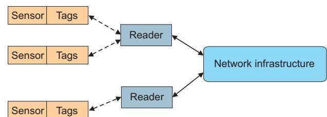
**Fig. 1.** An Overview of an EPC Network. The arrows indicate the flow of data from tags to network support system and the flow of control and data back to the Readers and tags.
