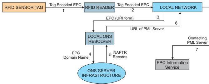
**Fig. 7.** An overview of an ONS system functionality [13]. An EPC encoded in an RFID label is read by an RFID Reader where the different functionalities associated with the EPC or services provided by an EPCIS associated with the tag is resolved through a query of the local ONS server. In the event that the local ONS server is unable to satisfy the requests it is forwarded to a global ONS server for resolution.
