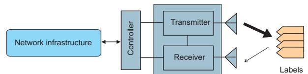
Fig. 4. RFID System overview. The transmitter, Receiver, and the Controller forms the RFID Reader. Here a transmitter of interrogation signals which is contained within a Reader communicates via electromagnetic waves with an electronically coded label to elicit from the label a reply signal containing useful data characteristic of the object to which the label is attached. The reply signal is detected by a receiver in the interrogator and made available to a control system.
