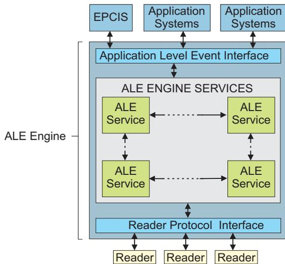
Fig. 6. Architecture of a ALE Engine System and its interaction with EPC Network components; EPCIS and Readers [11].
