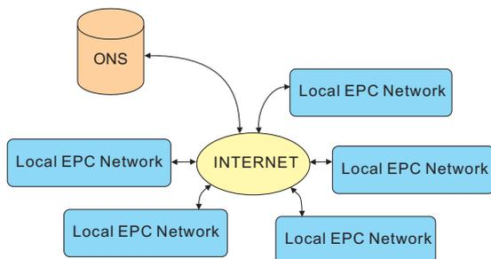
Fig. 3. Wide area EPC Network overview. The local EPC networks are able to route their information and requests to remote and unknown locations using the translation services provided by a network of global public ONS servers.
