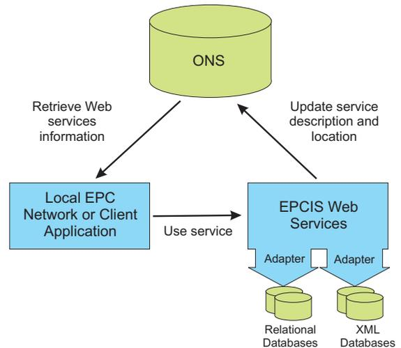
**Fig. 8.** Interaction between EPCIS, ONS and external applications
