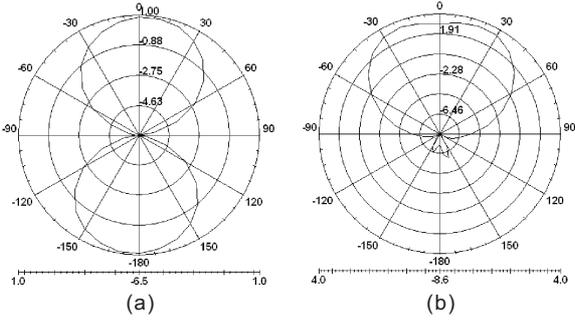
Figure 2: The  $yz$ -plane radiation pattern of the RFID tag antenna: (a) tag in free space; (b) tag located 3 mm above a  $1.5\lambda \times 1.5\lambda$  metallic plane (Antenna dimension:  $H_{rec} = 10$  mm,  $L_{rec} = 25$  mm and  $W_{rec} = 5$  mm).
