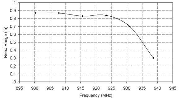
Figure 4: Read range measured over a frequency range
