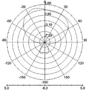
Figure 3: The  $yz$ -plane radiation pattern of the RFID tag antenna located 3 mm above a  $1.5\lambda \times 1.5\lambda$  metallic plane (Antenna dimension:  $H_{rec} = 10$  mm,  $L_{rec} = 25$  mm and  $W_{rec} = 15$  mm).
