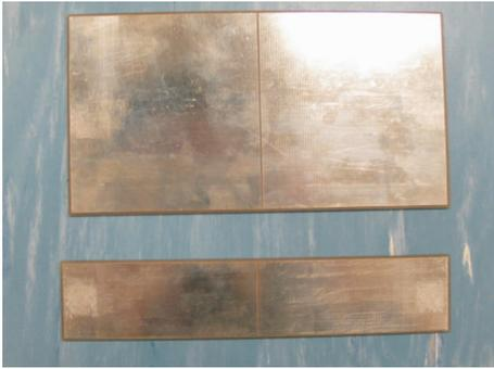
Fig. 5. The fabricated decouplers. The size of each patch of the narrow decoupler is 76mm(L)×30mm(W). The size of each patch of the wide decoupler is 78mm(L)×80mm(W). The slit width  $s$  is 0.5mm in both cases.
