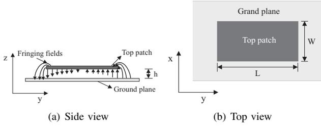
Fig. 3. The structure of a simple rectangular patch antenna without excitation.
