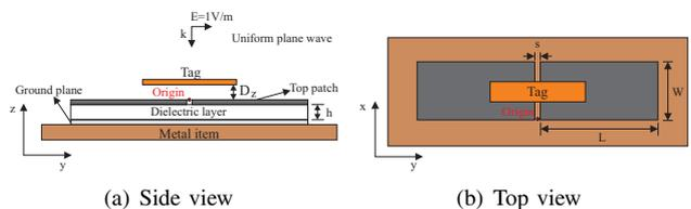
Fig. 1. Slitted decoupler structure illustration. A tag is placed above the slitted decoupler in a distance  $D_z$ . Below the decoupler, can be seen the metal item.
