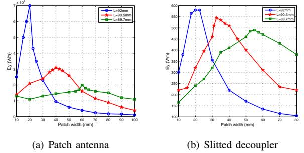
Fig. 4. The  $y$ -directed electric fields as a function of the patch width at various patch length. The thickness of dielectric layer  $h=1\text{mm}$ ,  $E_y$  is the magnitude of the r.m.s. phasors of the  $y$ -directed electric fields on the patch edge of patch antenna for sub-figure(a) and in the slit of slitted decoupler for sub-figure(b). For sub-figure(b), the width of slit  $s=0.5\text{mm}$ .
