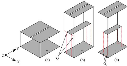
Fig. 2. (a) Standard cavity-backed slot antenna. (b) Miniaturized step 1. (c) Miniaturized step 2.
