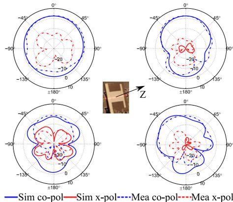
Fig. 5. Simulated and measured realized gain (dBi) patterns for free space (top row) and on-body (bottom row). Left column is  $zy$  plane and right column is  $zx$  plane.
