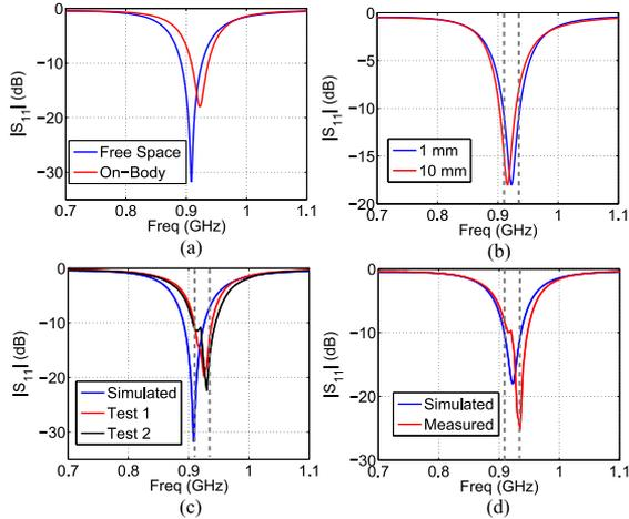
Fig. 3. (a) Simulated reflection coefficient in free space and on-body, (b) simulated reflection coefficient on-body with 1- and 10-mm spacing, (c) simulated and measured free-space reflection coefficient, and (d) simulated and measured on-body reflection coefficient.
