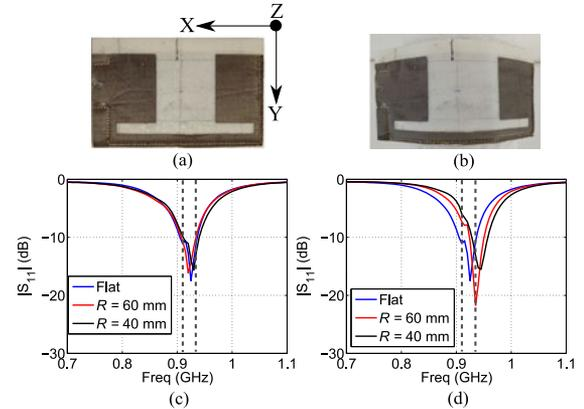
Fig. 4. (a) Antenna in flat state, (b) antenna bent along  $y$ -axis, (c) measured bending reflection coefficient in  $zy$  plane, and (d) measured bending reflection coefficient in  $zx$  plane.
