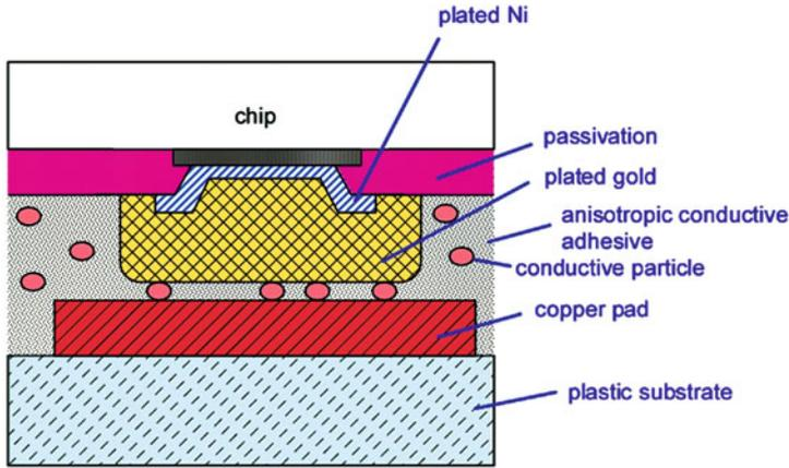
**Fig. 2** Anisotropic Conductive Film (ACF) circuit attach
