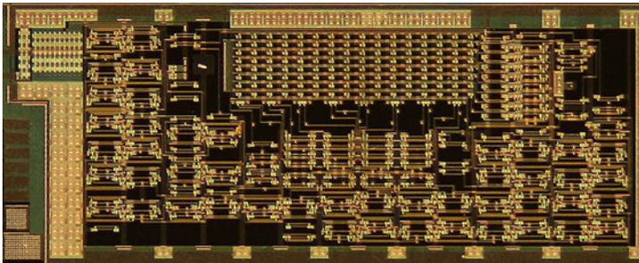
**Fig. 1** Printed IC with circa 1000 TFT devices (Photograph courtesy of Kovio Inc. © Kovio Inc.)
