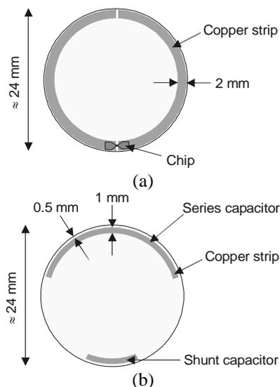
Fig. 4: (a) Front view; (b) Rear view of the sheep ear tag
