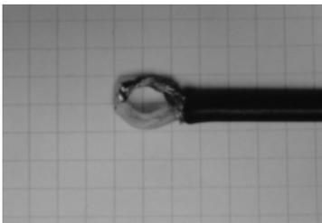
Fig. 5: A simple small loop used to determine resonance point of RFID tag
