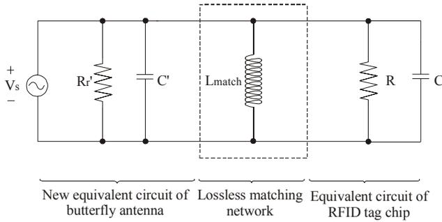
Fig. 4: Simplified circuit of RFID tag with a simple matching network
