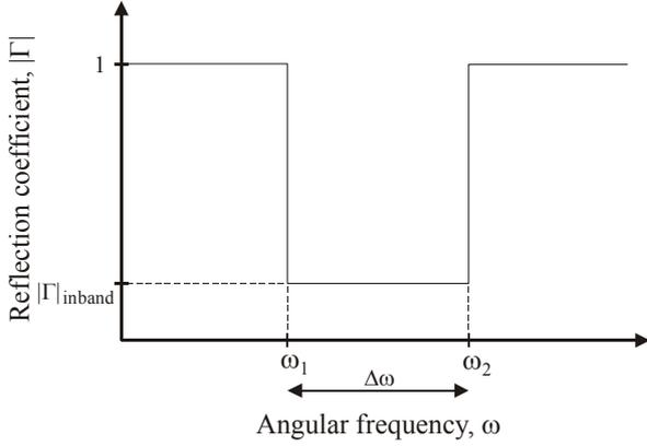
Fig. 2: Reflection coefficient for best utilisation of  $\pi/(RC)$ .
