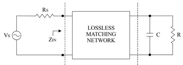
Fig. 1: A circuit with a lossless matching network and a parallel RC load
