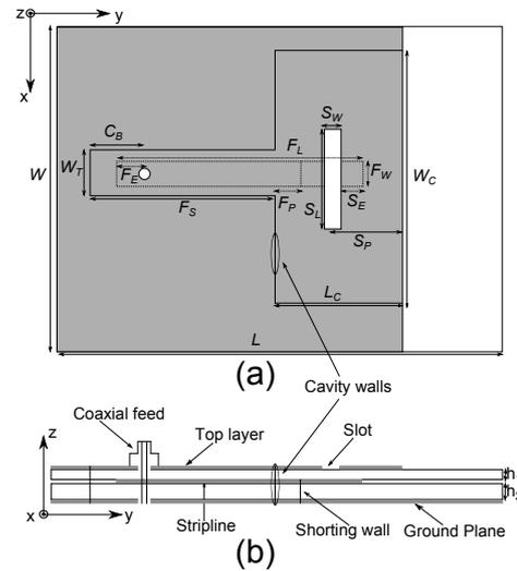
Fig. 1: Geometry of proposed antenna (a) Top View, (b) Side View. The optimized parameters are  $C_B = 4$  mm,  $F_E = 2$  mm,  $W_T = 12$  mm,  $F_S = 20$  mm,  $W_C = 81.5$  mm,  $L_C = 35.5$  mm,  $F_P = 9$  mm,  $F_L = 40$  mm,  $F_W = 6$  mm,  $S_L = 18$  mm,  $S_W = 1$  mm,  $S_E = 5.2$  mm,  $S_P = 18$  mm,  $h_1 = 1.6$  mm,  $h_2 = 3.2$  mm,  $W = 100$  mm,  $L = 95$  mm
