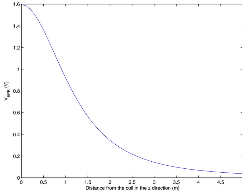
Figure 13: Turn-on range of the theft detection tag (measured from a “screaming corridor”).
