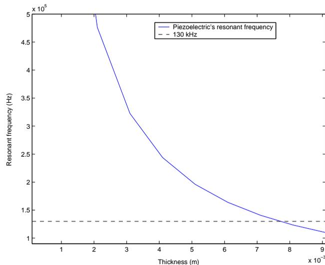
Figure 10: Resonant frequency of a PZT ceramic as a function of its thickness.
