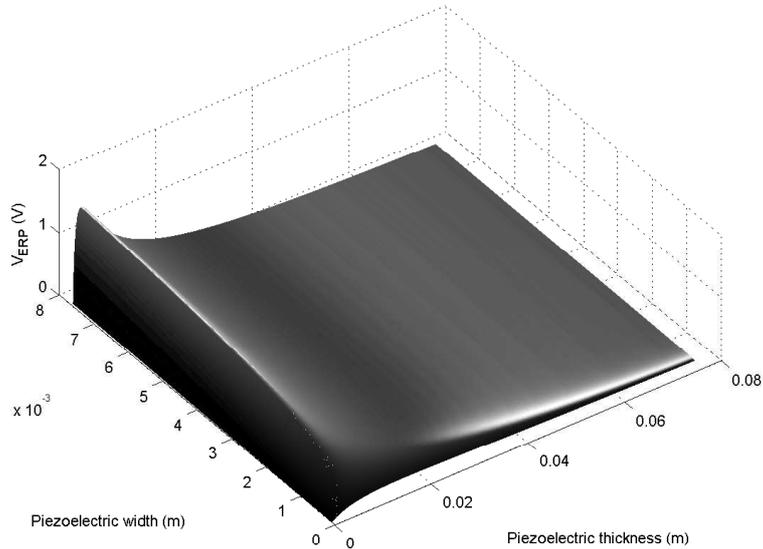
Figure 11: Effect of the piezoelectric structure dimensions on  $V_{EPR}$  at  $z = \frac{1}{2}$  meter from the “screaming corridor”.
