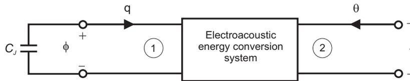
Figure 8: Representation of the electroacoustic energy conversion system with an electrical load.
