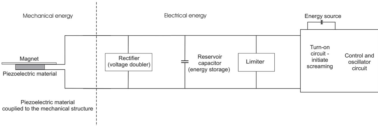
Figure 2: Components of the theft detection system.
