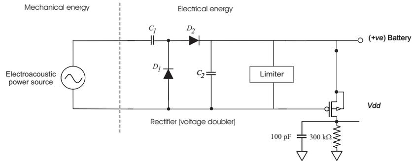
Figure 9: MEMS based theft detection turn on circuit schematic
