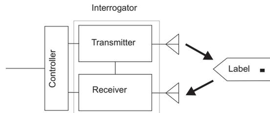
Figure 1: Illustration of an RFID system.
