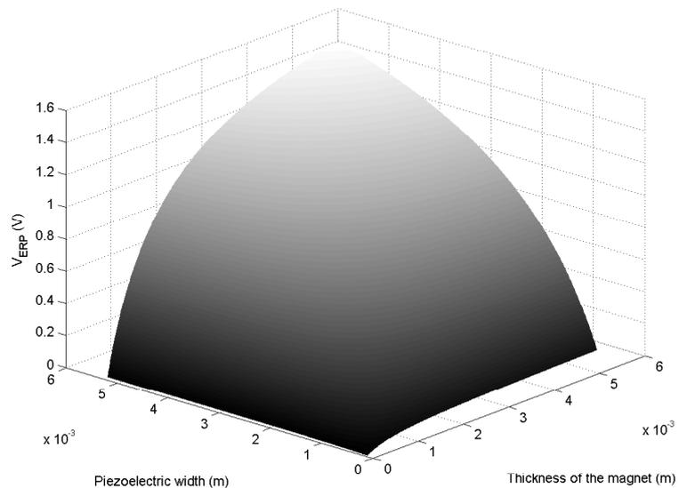
Figure 12: Effect of the magnetic structure dimensions on  $V_{EPR}$  at  $z = \frac{1}{2}$  meter from the “screaming corridor”.
