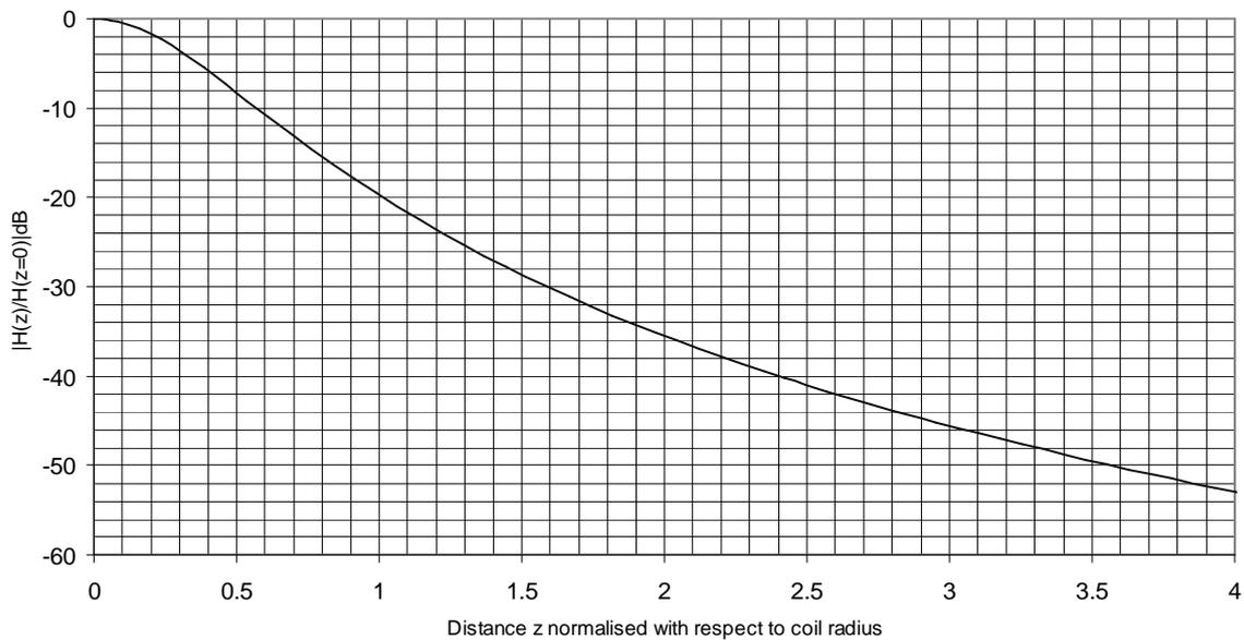
Figure 5: Relative magnetic field strength at a normalised distance ( $z/a$ ) from a circular coil
