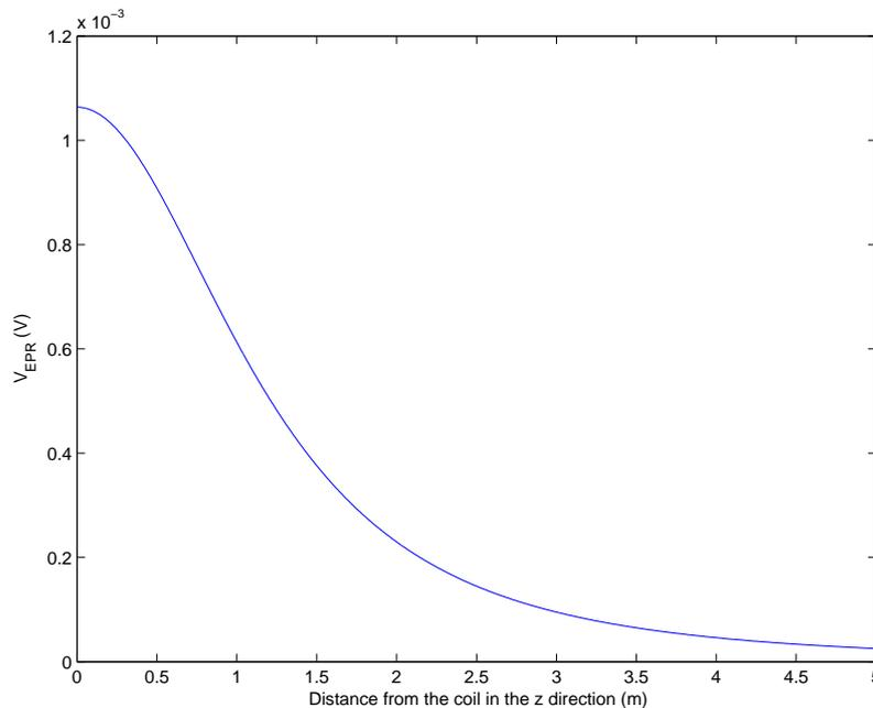
Figure 14: Turn-on range of the theft detection tag (measured from a “screaming corridor”).
