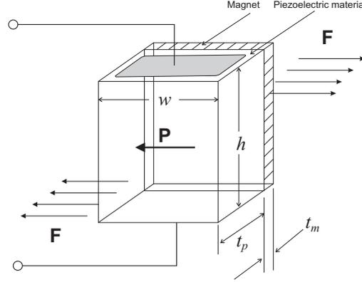
Figure 7: Magnet coupled to the piezoelectric material. Here  $\mathbf{F}$  is the shearing force applied by the magnet and  $\mathbf{P}$  is the direction of polarization of the piezoelectric material
