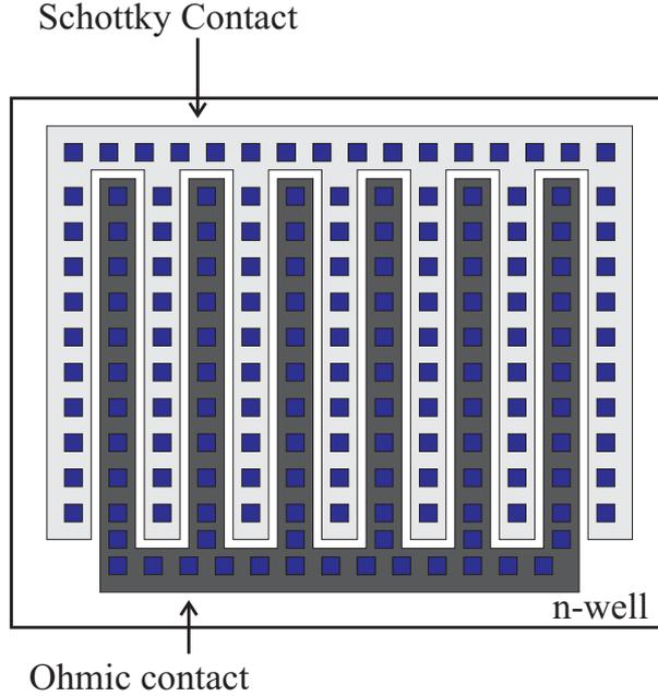
**Figure 7.** Top view of multi-finger Schottky contact diode.
