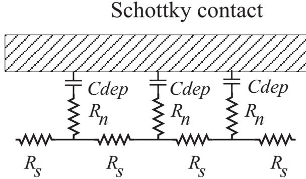
**Figure 4.** Diagram, illustrating the distribution nature of the resistance and capacitance of the Schottky contact.
