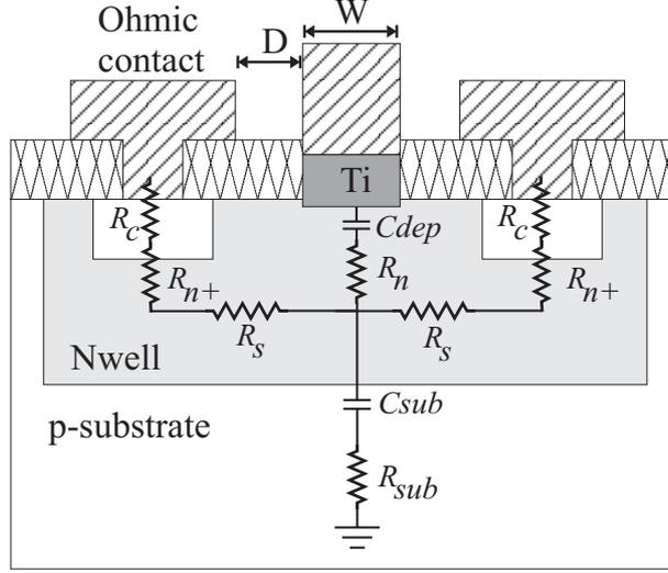
**Figure 3.** Equivalent circuit of Schottky diode, illustrating the various components of the series resistance.
