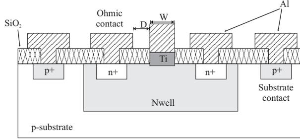
**Figure 2.** Cross sectional view of a planer Schottky Barrier Diode.
