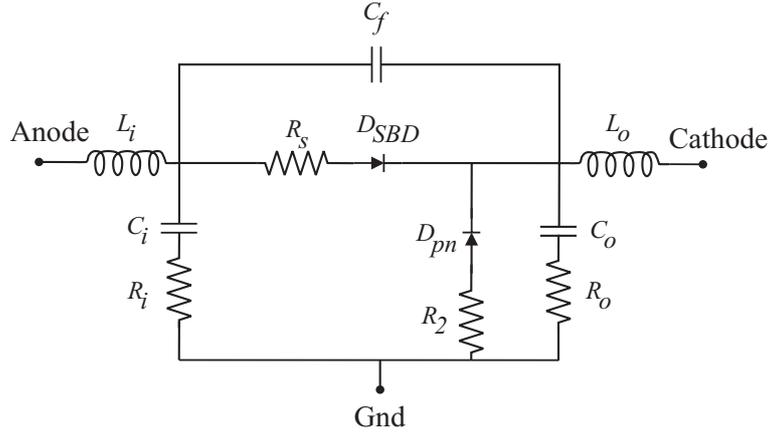
**Figure 6.** Equivalent circuit model of a Schottky Diode.
