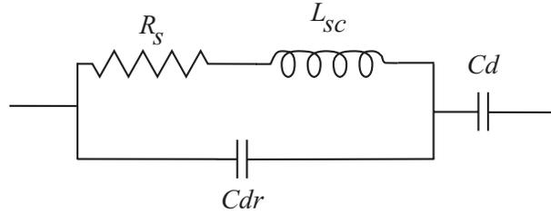
**Figure 5.** Equivalent circuit model of a Schottky diode that includes the effects of the displacement capacitance.
