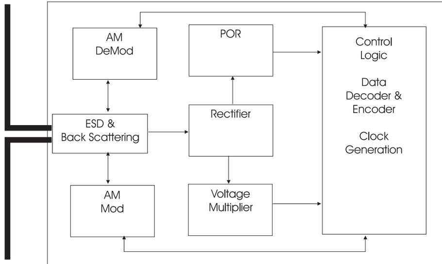
**Figure 1.** Architecture of a transponder RFID IC.
