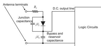
Fig. 1 RFID label schematic.
