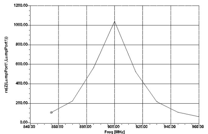
Fig. 3: Simulated real part of antenna impedance (ohms vs. MHz).
