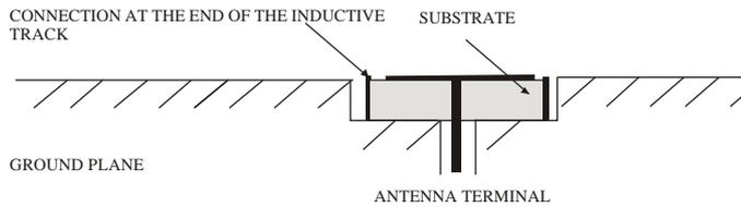
Fig. 1 Antenna structure (planar view)
