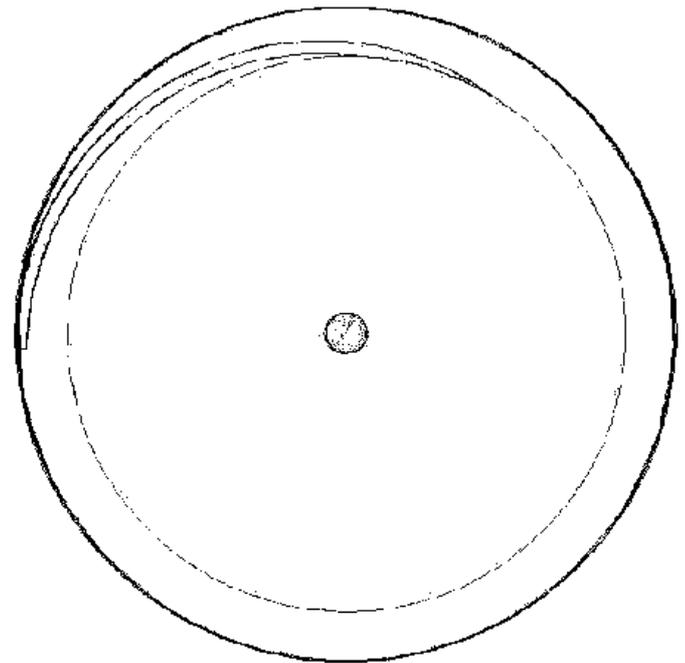
Fig. 2: Outline of the plate antenna, showing inductive track connecting centre plate to surrounding tub metal (top view).
