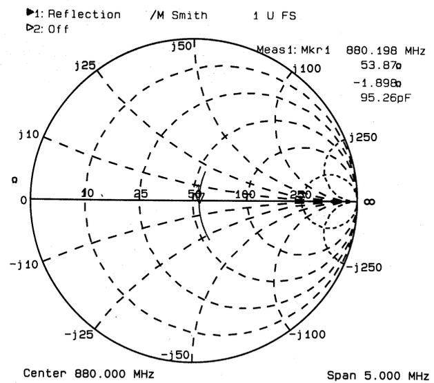
Fig. 8: Measured antenna impedance.
