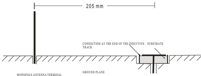
Fig. 5: Measurement arrangement.
