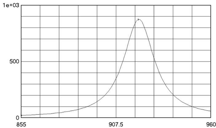
Fig. 6: Measured real part of antenna impedance (ohms vs. MHz).
