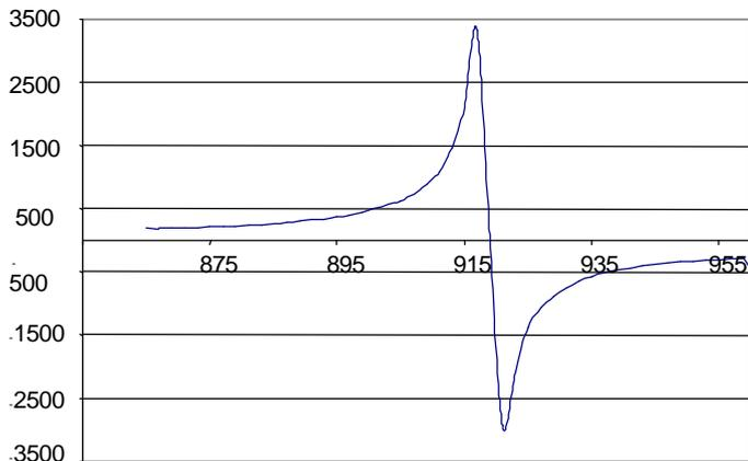
Fig. 7: Measured reactance of antenna impedance (ohms vs. MHz).
