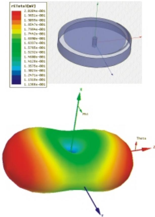
Fig.4: 3D Polar plot of the radiation pattern obtained from simulations.
