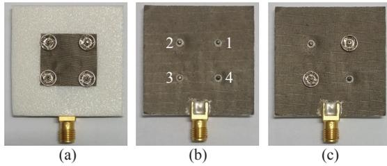
Figure 4: The antenna realization. (a) Top view. (b) Bottom view without female snap-on buttons (no shorts to the ground). (c) Bottom view with engaged female button at corners 1 and 3.
