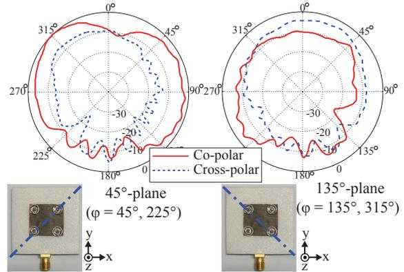
Figure 6: The measured normalized radiation patterns of the antenna in the 45°- and 135°-plane at 3.6 GHz. The diagonal dotted lines on the antenna indicates the 45°- and 135°-planes. Corners 1 and 3 were shorted in this antenna configuration.
