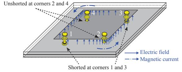
Figure 2: Electric field distribution of the antenna with engaged shorting vias at corners 1 and 3.
