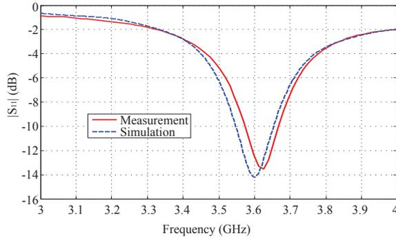
Figure 5: Measured and simulated  $|S_{11}|$  of the antenna.
