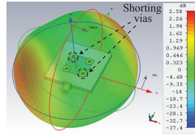
Figure 3: The simulated 3D gain pattern in CST Microwave Studio 2016.
